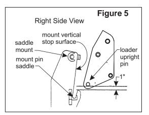
11. Remove hoist chain or strap from loader boom and secure to each bucket cylinder shipping brackets (D) (see figure 3). Using overhead hoist raise front of loader to rotate loader upright into upper mount saddle (see figure 6). Continue to rotate loader upright until upright has fully seated into back of mount saddle. Insert two 1-1/4" x 7" pins (F) and linch pins (E) which were removed from loader uprights in step 3 (see figure 7). Remove hoist chain or strap from shipping brackets.
