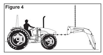
**NOTE:** It is important to attach lift cylinder hoses (yellow and green spiral band coded) for loader to function properly. Do not connect boom oil line hoses for tilt cylinder control at this time. (Connect these after shipping brackets are removed from attachment pin hubs instruction 12)
