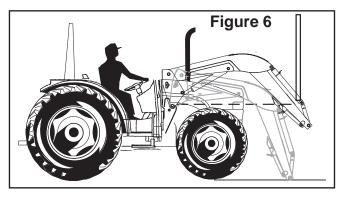
**NOTE:** In some cases a small amount of additional force may be required to insert the pins. If necessary, use a drift and hammer made of non- sparking material (a shot-filled mallet is recommended) to seat loader uprights into mount saddle.
