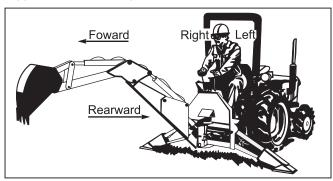
**NOTE:** References to right, left, forward and rearward directions are determined from the backhoe operator seat position facing rearward.
