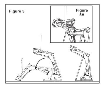
**NOTE:** Do not over tighten lock nut (A). Parking stand tube must pivot freely.
