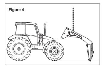
**NOTE:** Install valve kit or hose kit onto tractor before proceeding to instruction 5 on page 6.
