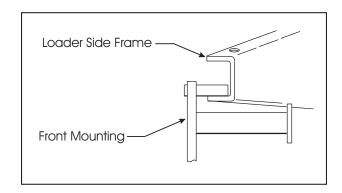
**NOTE:** Lower lip of loader side frame channel must be between front mounting tubes.
