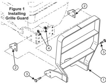
**NOTE:** Do not use spacers (2) if tractor is equipped with a mower deck. Fasten grille guard and mower deck front hanger brackets to tractor frame in place of spacers (2).
