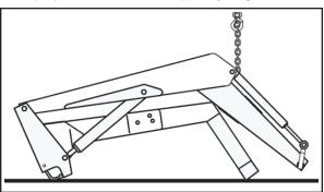
**NOTE:** Snug hardware connecting yoke to loader side frames, but do not torque completely. After loader has been mounted to tractor and aligned with mid mounting brackets and front mounting brackets, torque hardware to 262 ft.·lbs.
