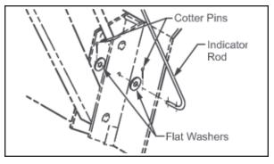
3. Locate tractor and loader on level surface. With bottom of attachment resting on surface, cut off excess rod flush with end of guide tube or paint exposed rod a contrasting color.
