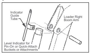
Slide level indicator rod through guide tube. Attach
