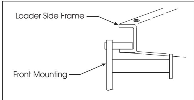
4. Clamp hinges around midmounting tubes using hardware provided.
