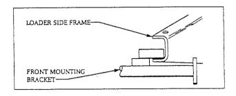
3. Attach lift boom frame and lift boom cylinders to side frame uprights with 1" x 4-3/8 pins, 3/8 x 1" shoulder bolts and lock nuts. Center loader on mid mounting bracket tubes and tighten hardware clamping hinges around tubes of mid mountig bracket
