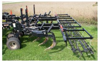
In addition to being available for new 10 Series EarthMasters, the new harrow attachments can be retrofitted onto existing 100 Series machines, the 1700, 2200 and 2200F, and the 2500. This ability to retrofit may enhance the value of your dealer's used machines since it allows him to match his used machines to his customers' field surface finish requirements.
